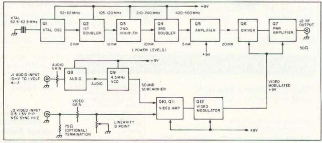
Figure 1. Video transmitter block diagram.
